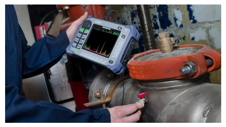
The EPOCH 650 digital ultrasonic flaw detector combines Olympus' industry-leading conventional flaw detection capabilities with the efficiency of a highly portable, intuitive instrument. The EPOCH 650 flaw detector's blend of efficient menus and direct access keys enables you to take advantage of the highest quality flaw detection platform with exceptional ease of use.
