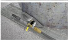
3. Connect vacuum pump or compressor hose to begin vacuum test.
