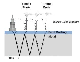
With Multiple-Echo, readings are taken by measuring the time delay between any three consecutive backwall echos. The time of T1 (coating thickness) is ignored. The times of T2 and T3 are equal to the time that it takes to travel through the metal. Only by looking at three echoes can the measurements be automatically verified (where T2 = T3).
