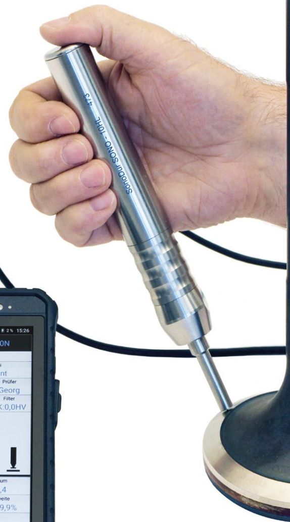
Handheld Probe SONO-10HL "long nose" used on valve head
